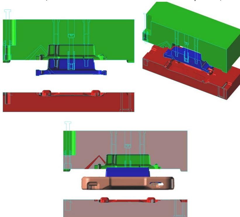
External/male undercuts are not possible due to the expansion process; the self-ejecting forces create tooling release issues.
