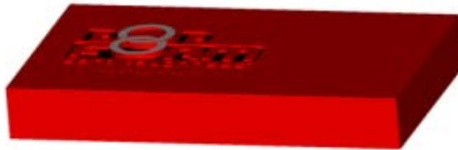
Parts without draft cannot eject from the mold
