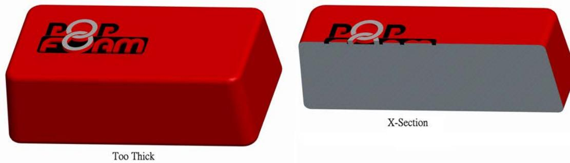
Coring removes material from the part which can allow for faster cycle times which reduces the overall cost of the part.
